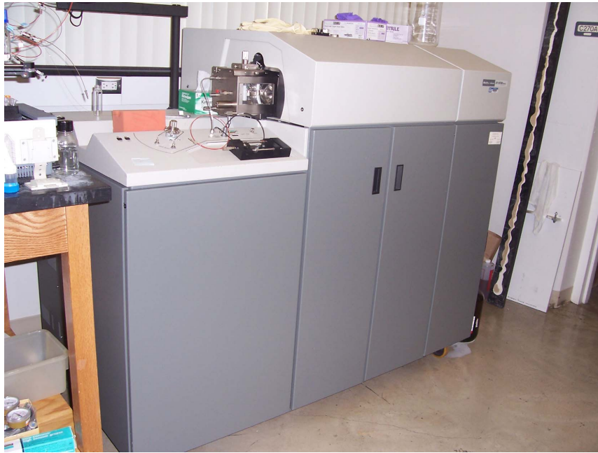
Figure 2.2: The Qstar Pulsar i ESI-LC TOF Mass Spectrometer used at BYU
